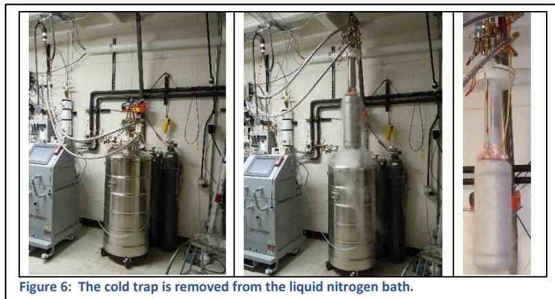
Figure 6: The cold trap is removed from the liquid nitrogen bath.
