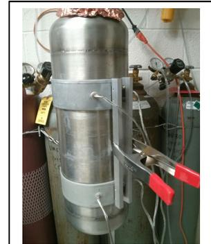
Figure 7: Two band clamp heaters quickly warm the cold trap and prevent excessive icing during regeneration.
