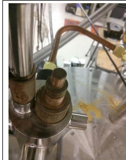
Figure 29: The top view of an Oxford 8T magnet showing the magnet current leads and pressure equalization tubes (copper).
