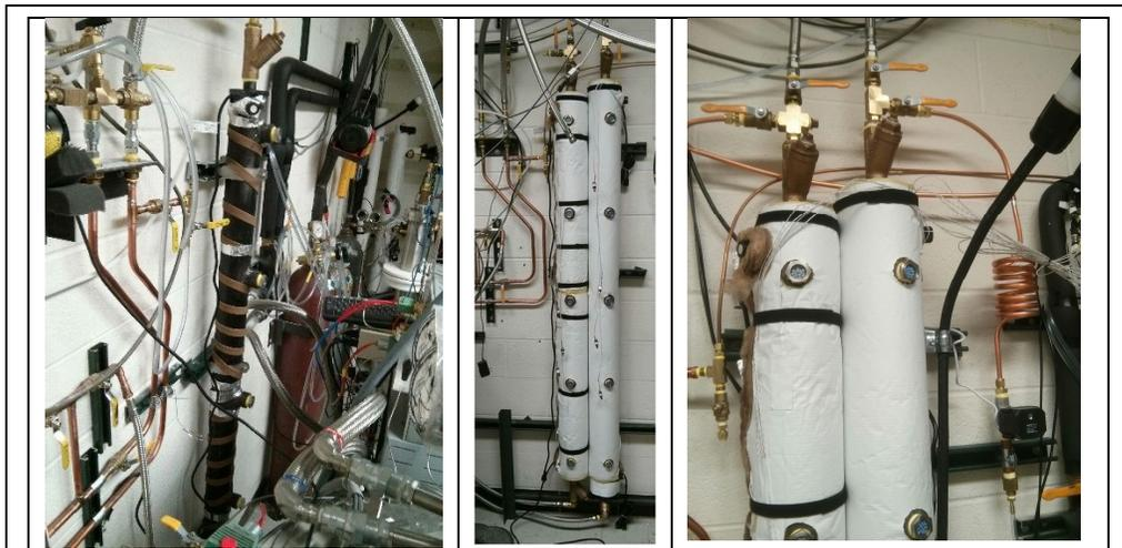
**Figure 5:** The water traps are filled with activated alumina. (left) A water trap with the fiberglass insulation removed reveals the silicone heater tapes and thermostats. (center) The two traps are mounted side-by-side. (right) Helium gas enters the top of the traps and exits the bottom. During regeneration, a counter flow of air enters the bottom of the trap and exits the top of the trap. This exhaust gas is routed through a cooling coil and then a motorized ball valve.
