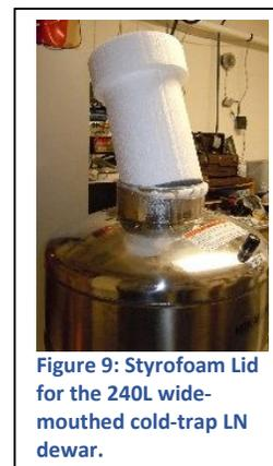
Figure 9: Styrofoam Lid for the 240L wide-mouthed cold-trap LN dewar.
