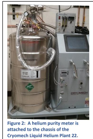
Figure 2: A helium purity meter is attached to the chassis of the Cryomech Liquid Helium Plant 22.
