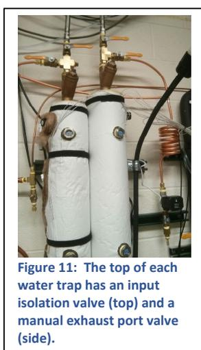
Figure 11: The top of each water trap has an input isolation valve (top) and a manual exhaust port valve (side).
