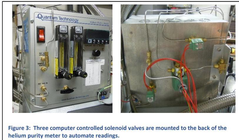
Figure 3: Three computer controlled solenoid valves are mounted to the back of the helium purity meter to automate readings.
